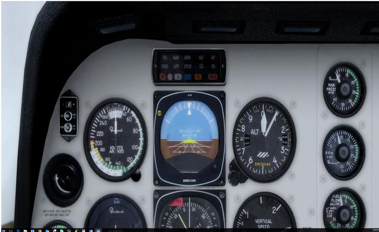
In this case I specified top and bottom SideAngles of 10.0 and -10.0 degrees (a vertical FOV of 20 degrees) which is observably much too small of a vertical FOV angle for things to look right.
